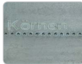
Punching with variable penetration
