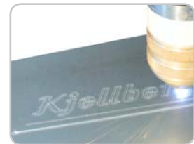
Marking with adaptable line width and depth
