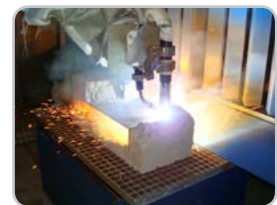
HotWire-cutting of non-conductive materials
