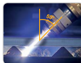
Bevel cutting with an angle of 50°
